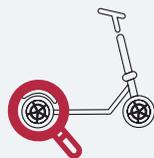
\* Metal vibration may occur due to motor vibration, vibration of the brake disc and pad during the load section that accelerates during driving. (About 15 - 30Km, different for each product)
