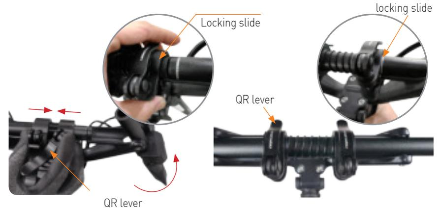
3. Handlebar unfolding
